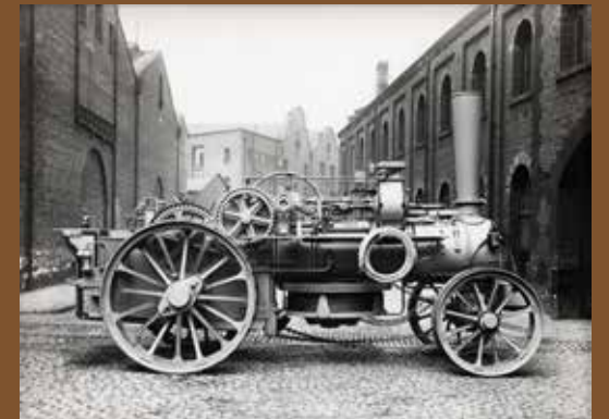
A completed Fowler steam ploughing engine fresh off the production line, around 1900.
